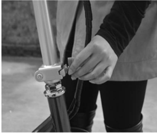
Step 4: Tighten the handle quick lock sleeves
