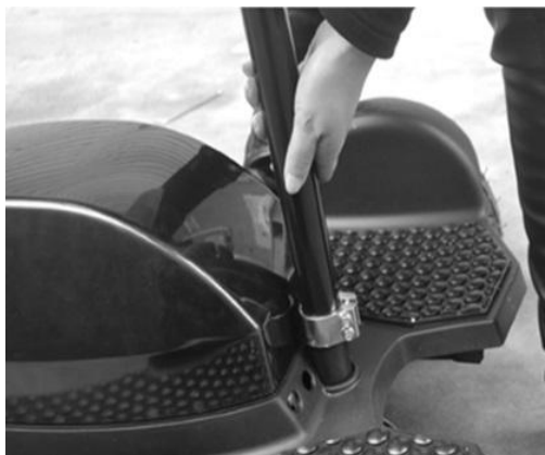
Step 6: Insert the seat rod, and tighten the screws
