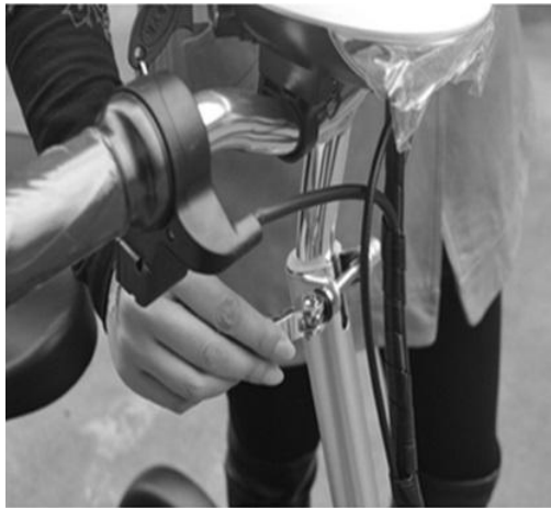
Step 5: Adjust the handlebar direction first, then buckle up the quick lock
