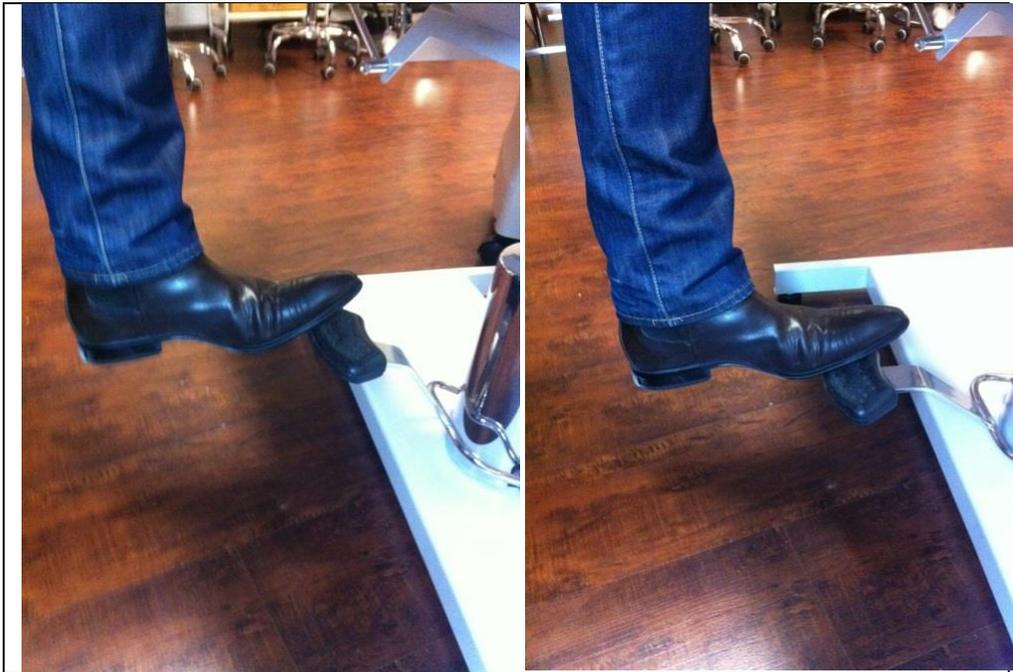
2) Press pump all the way down to release the pump and Lower the Height.
